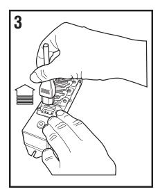
To remove the connector, depress the thumb tab and hold down while extracting the connector from the inlet or outlet.
