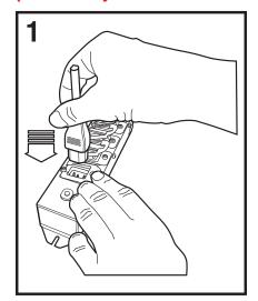
Depress the thumb tab and fully insert the connector into the inlet or outlet.
