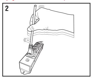
Release the thumb tab which will automatically engage the lock, holding the connector in place.
