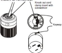
NOTE: DO NOT back out terminal screws completely. Could cause damage when threading screws back into terminals.
