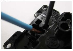
2) Apply downward pressure in the square aperture to open the terminal clamping spring and hold in the open position. Slide wire into open terminal, making sure insulation goes in beyond the lip of the round aperture (see photo below).
