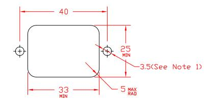
Note 1: Recommended diameter for thru-hole (screw/nut combination) hardware mounting method. Other methods will require holes with different dimensions and parameters.
