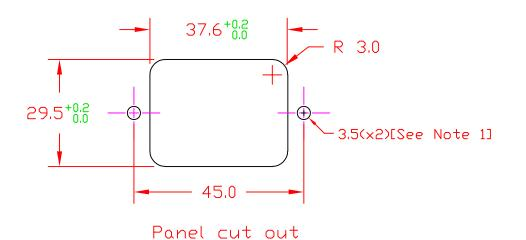
Note 1: Recommended diameter for thru-hole (screw/nut combination) hardware mounting method. Other methods will require holes with different dimensions and parameters.
