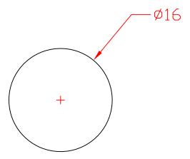
Suggested Clearance Hole for Non-Threaded Mounting
