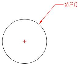
Suggested Clearance Hole for Non-Threaded Mounting
