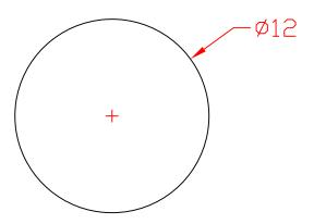
Suggested Clearance Hole for Non-Threaded Mounting
