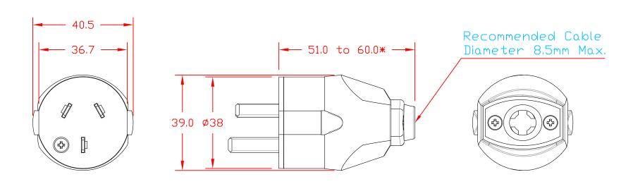
\* Cable diameter will vary length of part based on cable entry/clamping design.
