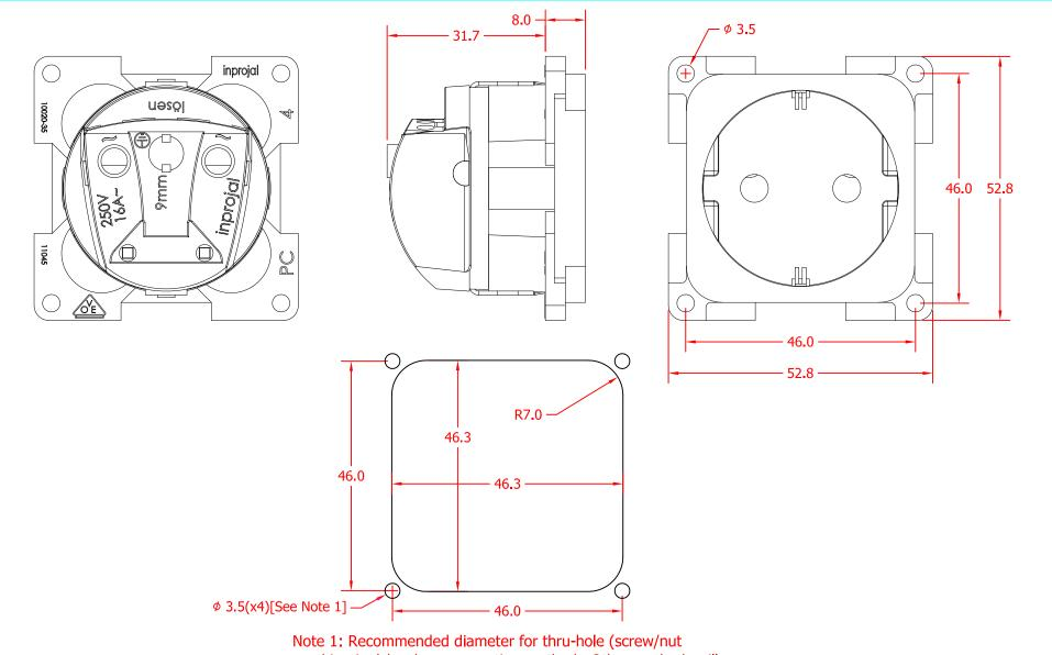
Note 1: Recommended diameter for thru-hole (screw/nut combination) hardware mounting method. Other methods will require holes with different dimensions and parameters.
