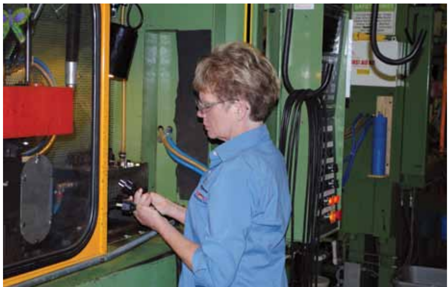
Visual inspection of the Schuko plug after molding
